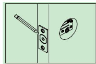
b.Chisel  $1/8''$  (3mm) deep along the outline to allow the faceplate to be aligned with the door edge.
