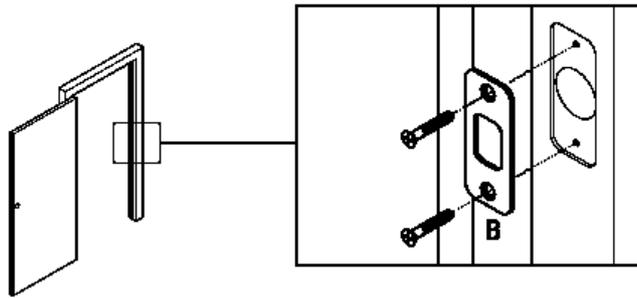
3. Locate center of strike hole by measuring back from door stop, 1/2 the thickness of door.
