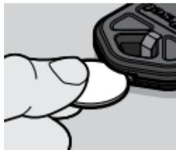
2、 Remove the square board and battery assembly, and keep the gasket in the bottom half of the fob.
