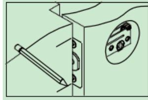
b. Chisel 5/64" (2mm) deep along the strike outline to allow the strike to be aligned with the doorframe.
