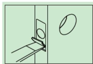
c.Insert the latch and tighten it with screws.Note : please use tapping screws for metal door.
