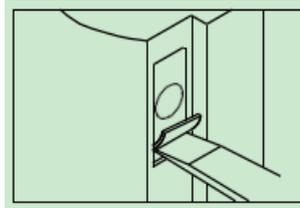
c. Insert the strike and tighten it with screws. Note : please use "tapping screws" for metal door.
