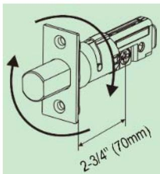
The BACKSET is the distance between the center of cross bore and edge bore of the door. Adjustable latch fits both BACKSET of 60mm (2-3/8") and 70mm(2-3/4"). Please follow the steps shown below for BACKSET adjustment.
