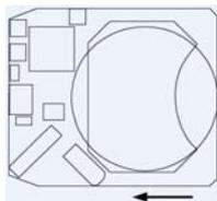
5. Place the square board and battery assembly back into the gasket, making sure that the side of the square board with the LED and button face the gasket.
